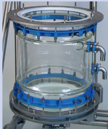
Heating / Cooling jacket Heiz- / Kühlmantel
